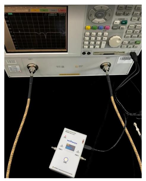
WACM will start system boot sequence if USB connected to VNA and it will take about 35 seconds.
