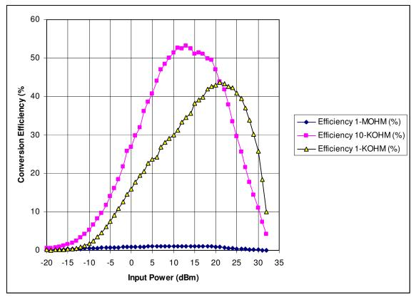
Figure 4. RF-DC conversion efficiency versus input power at 915MHz using the RFD102A mounted on the test board into 1-MOhm, 10-kOhm and 1-kOhm loads.
