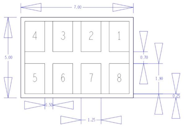
Figure 6. Module footprint. Dimensions are in millimeters. Pin 1=DC Output, Pin 4=RF Input, Pins 2,3,5,6,7,8=GND.
