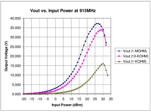
Figure 3. Output voltage versus input power at 915MHz using the RFD102A mounted on the test board into 1-MOhm, 10-kOhm and 1-kOhm loads.
