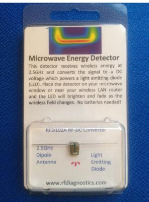
Figure 5. Microwave energy detector created using the RFD102A, a two-wire dipole and a surface mount LED.
